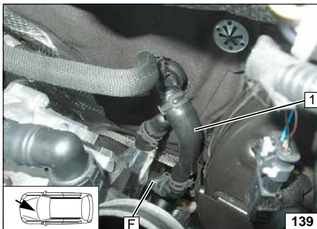
1 Heat exchanger inlet hose section
