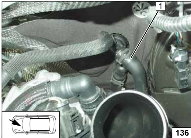
1 Hose of engine outlet / heat exchanger inlet
