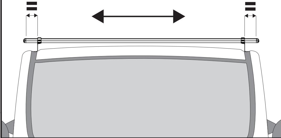
**5** Tighten the roof bar fixings to 8Nm.
