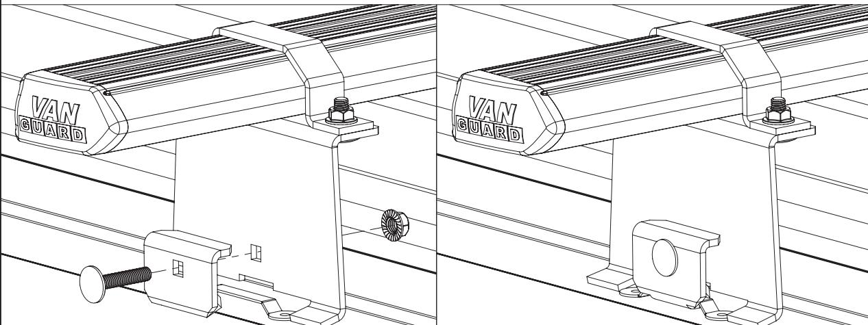
**4** Adjust the roof bars to ensure that they are evenly spaced on the vehicle.
