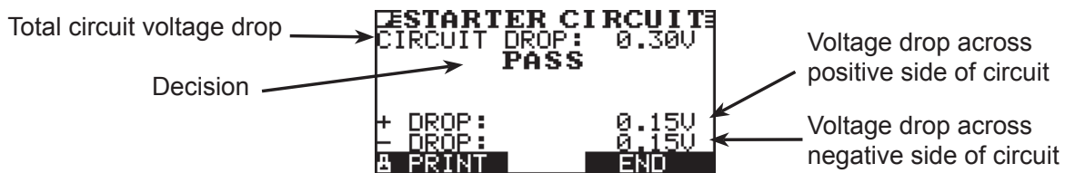
Figure 19: Starter Circuit PASS Result
