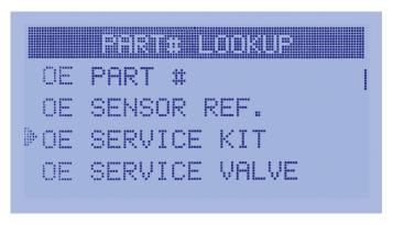
TPMS Go guides you to compatible sensors and part numbers for any vehicle, and indicates the correct torque values.
