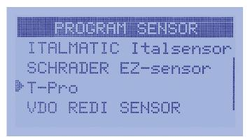
Quickly program aftermarket sensors, one wheel at a time. For relearning, use the TPMS Go with a diagnostic scan tool or follow the vehicle's instructions for auto or manual relearn.
