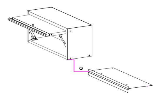
Step 3: To apply the 4pcs Phillips M6 Screw from inside the Cupboard Unit to the Support Bracket to secure the structure. Meanwhile, the plate cover is placed between the panel and the cupboard.
