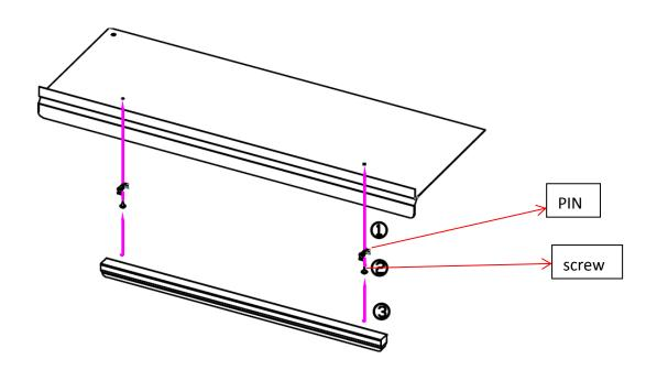
Step 2: To press the plate cover into the cupboard first.
