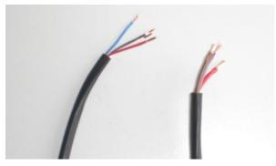
Remove max. 5 mm insulation from the wires of the "old" wiring harness that has been installed inside the vehicle (to be connected to the adapter wiring harness).
