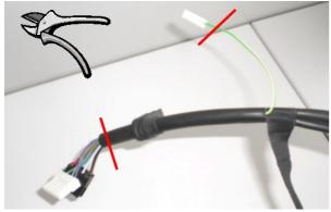
Cut off the plugs from the "old" wiring harness that has been installed inside the vehicle.
