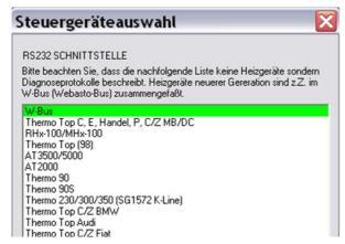
Connect Thermo Test PC-Diagnosis and check connection.
